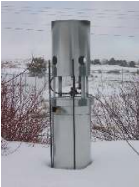
Figure 6: Manually Operated Silver Iodide Cloud Seeding Generator.
